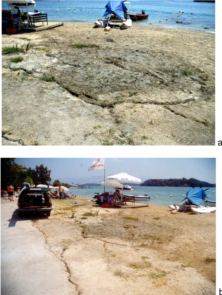
Fig. 9: Liquefaction and ground fissures at Nydri beach.
