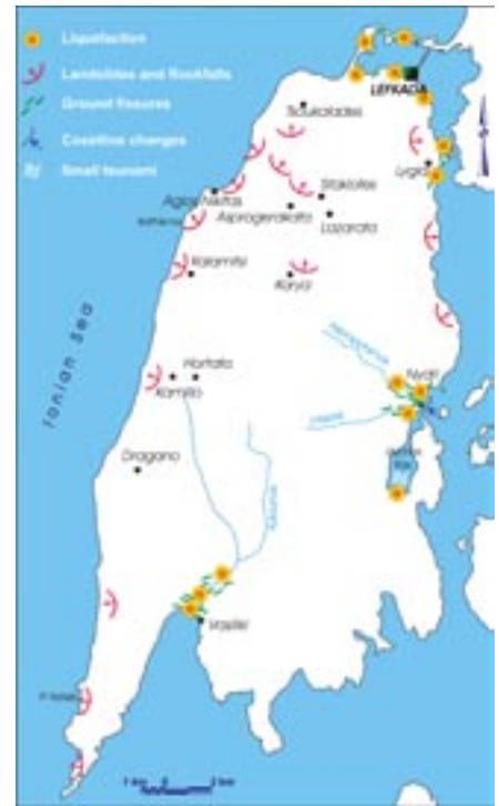
Figure 8. Geological and geotechnical effects of the Lefkada earthquake.
