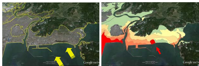
Figure 11: Protection lack in the area between the coastal forest and the port facilities in eastern Ishinomaki
